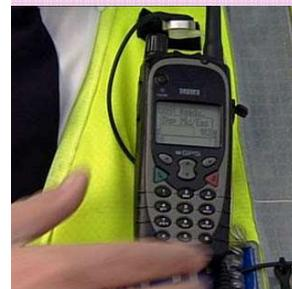
handset can double as a digital radio and mobile phone in one - and will also function as a data terminal. Officers can also talk directly to each other without the need to pass messages via the police control room.
